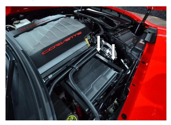
Remove fuse # 42 or #41 (2014) and insert the fuse in the open spot on the fuse tap as shown. Reinsert the fuse tap as shown with the fuse facing the passenger side fender. Using the utility knife make a tiny relief for the red and white wire to sit.
