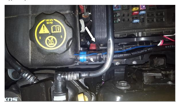
Attach the Ground wire as shown and use zip ties to secure it to the coolant line. Reinstall the fuse cover (make sure the wires are in the slot you created.
