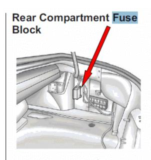
The rear compartment fuse block is located on the right side of the trunk behind a cover. Remove the convenience net retainers, the rear sill plate, and the passenger side trim retainers, then swing the trim out of the way.
